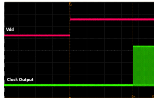
Figure 17. Startup Waveform vs. Vdd
