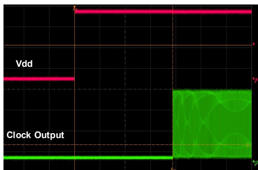
Figure 17. Startup Waveform vs. Vdd
